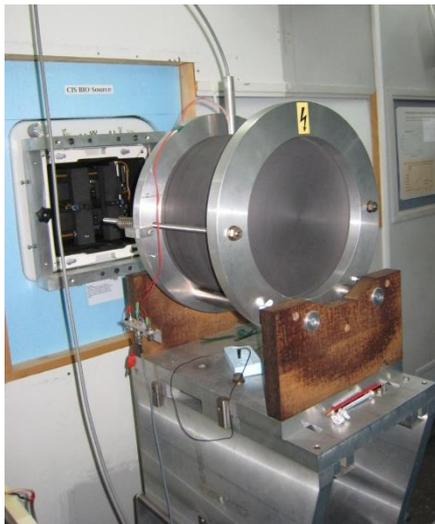
**Fig. 3-b** Photograph of the BIPM graphite phantom placed in the BIPM CisBIO Co-60 beam in 2011.
