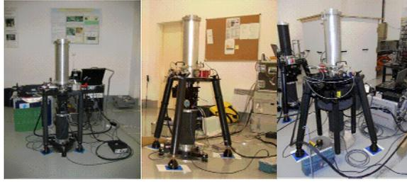
**Left)** FG5 Type New1 ( $C_{SAC} = -1.24 \pm 0.2 \mu\text{Gal}$ ), fiber laser optic interferometer with straight legs
